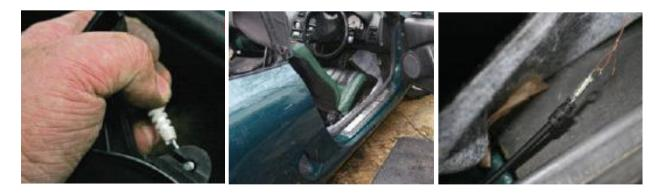
Feed the cable across the footwell and up, through into front bonnet area via a hole at the top of the footwell. Once the cable is through the grommet, it has to be pushed back into place. Clip the cable into place inside the front boot and fed through the last hole into the space beneath the slam panel.
