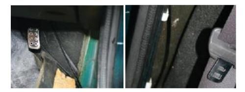
Lifting the carpet clear of the side of the cockpit reveals the cable route and the run of clips that are fitted to ensure it follows a set path, which it shares with the throttle cable and is clipped alongside. As you withdraw the cable make note of the path it takes and the clips that hold it down.
