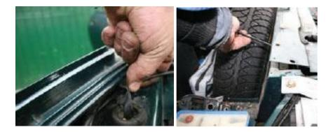
Clip the end of the new cable onto the latch assembly and push back into the space beneath the slam panel. The latch has captive nuts and it is quite easy to re-attach it to the slam panel. Before tightening the latch bolts it will be necessary to lower the bonnet and align the latch with the locking pin. Once they meet successfully the bolts can be fully tightened. Before shutting the bonnet have an assistant operate the lever to ensure it operates the latch effectively.
