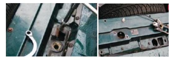
Once the latch is exposed the front end of the cable can be unclipped with the help of a pair of pliers. If the latch assembly is looking corroded and partly seized now is a good opportunity to give it a thorough wire brushing and lubricate all the moving parts liberally.
