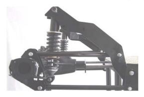
The conversion consists of parallel trailing arms, axle and body locating brackets, coil-over adjustable dampers and a panhard rod
