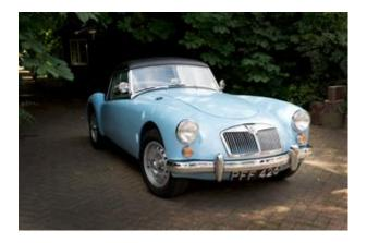
The standard axle ratio of 4.3/1 gives 17 mph per 1000 rpm in 4th gear. These characteristics give a very lively performance right up to maximum speed. The major drawback is apparent when cruising on motorways at 70mph for long periods.
