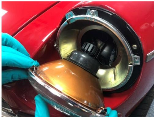
13. Holding the lamp in place reattach the retaining rim
