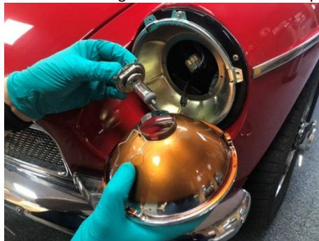
8. Taking a Q Parts LED light unit, slide off the clear protective sleeve. Holding the base of the lamp in one hand and the LED H4 locating plate in the other, gently twist the base of the lamp in an anti-clockwise direction to remove from the bayonet fitting.
