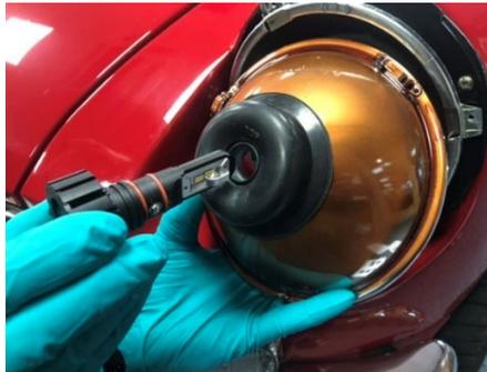
11. Connect the LED harness ensuring the arrows on each connector align before pushing together. Ensure the threaded portion abuts the o ring , then secure threaded collar.
