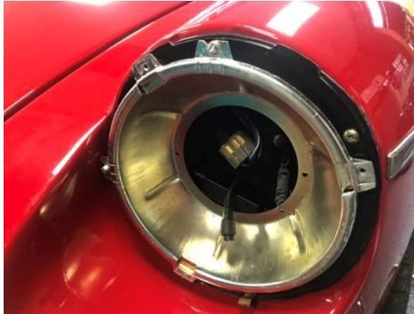
7. Remove weather-shield boot and existing H4 bulb from the headlamp
