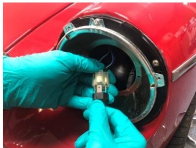
6. Locate the driver module close to the base of the inner bowl, this can be tucked under the retaining spring with the headlamp loom connection on the opposite side.
