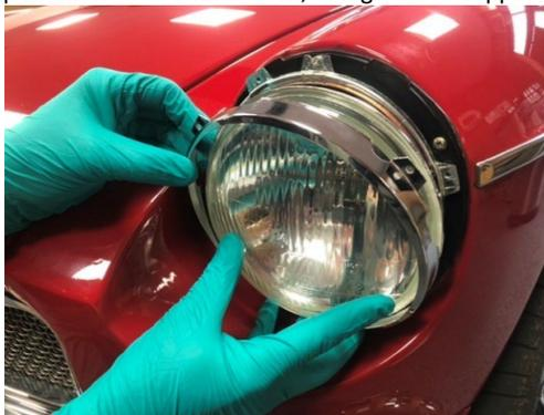
3. Remove the headlamp from the inner bowl to enable access to the rear.
