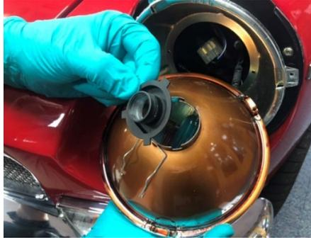
10. Examine the front of the lens and orientate so that the top of the lamp is in the twelve o'clock position. Taking the Q Parts LED light unit install into the headlamp, ensuring the trough like deflectors are at 6 o'clock position and twist the base in a clock wise direction to engage the bayonet fitting.
