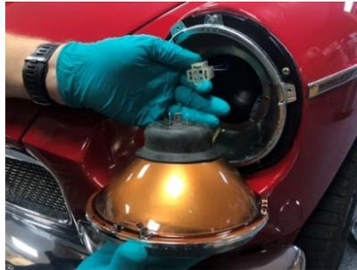
5. Remove a driver module from the packaging and attach the three pin male plug to the existing female block connector on the vehicles wiring loom, ensuring the connection is snug. Before continuing, **make sure there are no exposed electrical components** which could come into contact with the internals of the headlamp assembly (these should be insulated with electrical tape where necessary).
