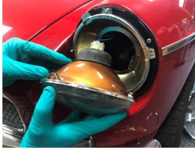
4. Disconnect the electrical connector block and if applicable, the pilot lamp from the headlamp and set the headlamp to one side.
