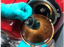
10. Examine the front of the lens and orientate so that the top of the lamp is in the twelve o'clock position. Taking the Q Parts LED light unit install into the headlamp, ensuring the trough like deflectors are at 6 o'clock position and twist the base in a clock wise direction to engage the
