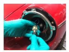
6. Locate the driver module close to the base of the inner bowl, this can be tucked under the retaining spring with the headlamp loom connection on the opposite side.
