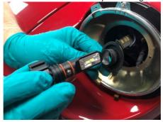
Locate the LED H4 locating plate within the rear of the headlamp and re-fit the wire retaining 9.
