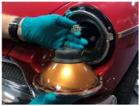
5. Remove a driver module from the packaging and attach the three pin male plug to the existing female block connector on the vehicles wiring loom, ensuring the connection is snug. Before continuing, make sure there are no exposed electrical components which could come into contact with the internals of the headlamp assembly (these should be insulated with electrical tape where necessary).
