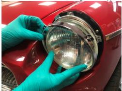
3. Remove the headlamp from the inner bowl to enable access to the rear.
