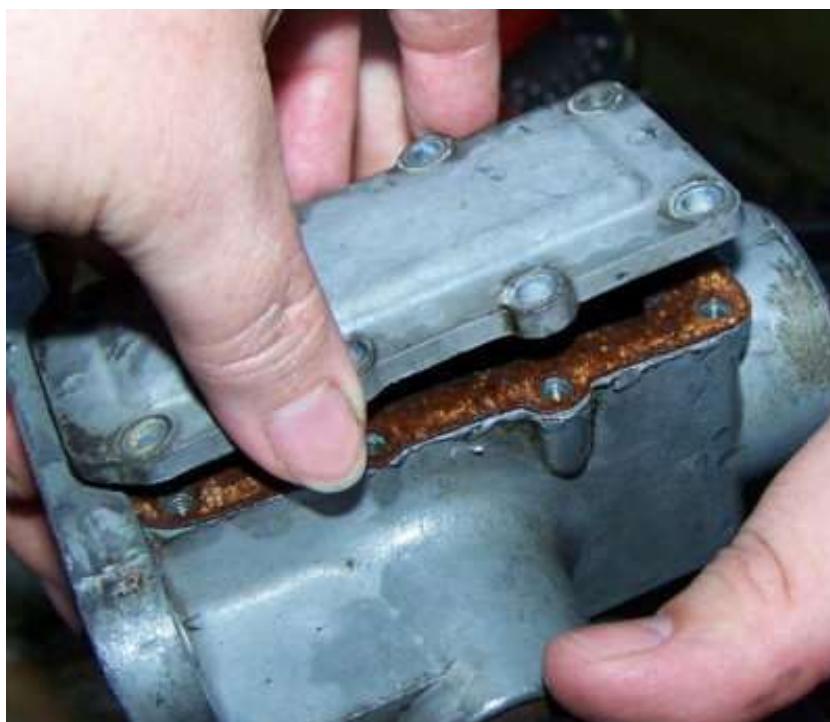
Replacing lever shock gasket and cover
