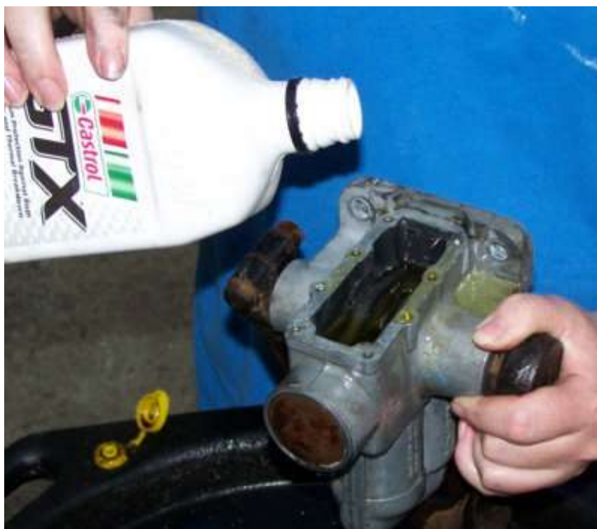
Rinsing lever shock with fresh engine oil
