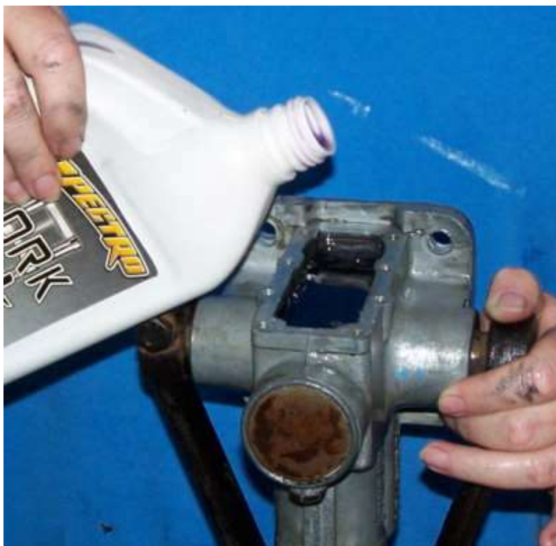
Refilling MGB Lever Shock with fork oil
