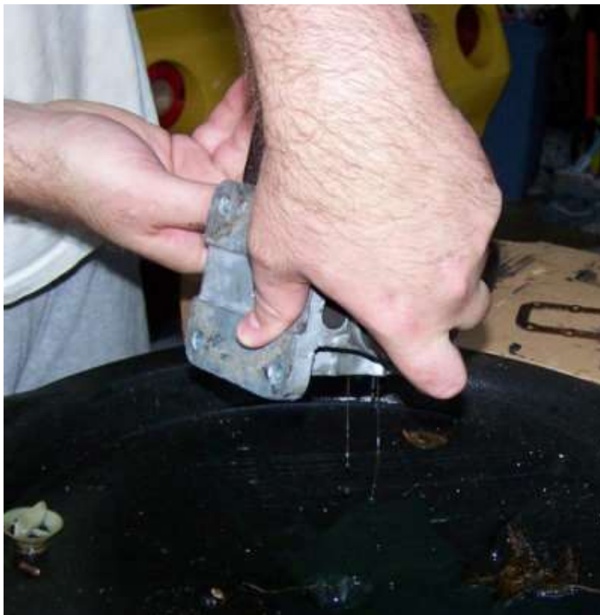
Draining oil from MGB lever shock
