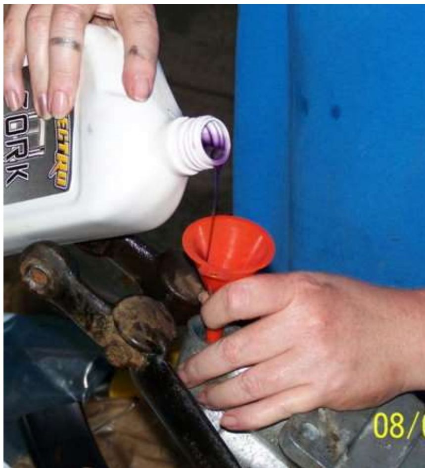
Topping up Armstrong lever shocks through valve opening
