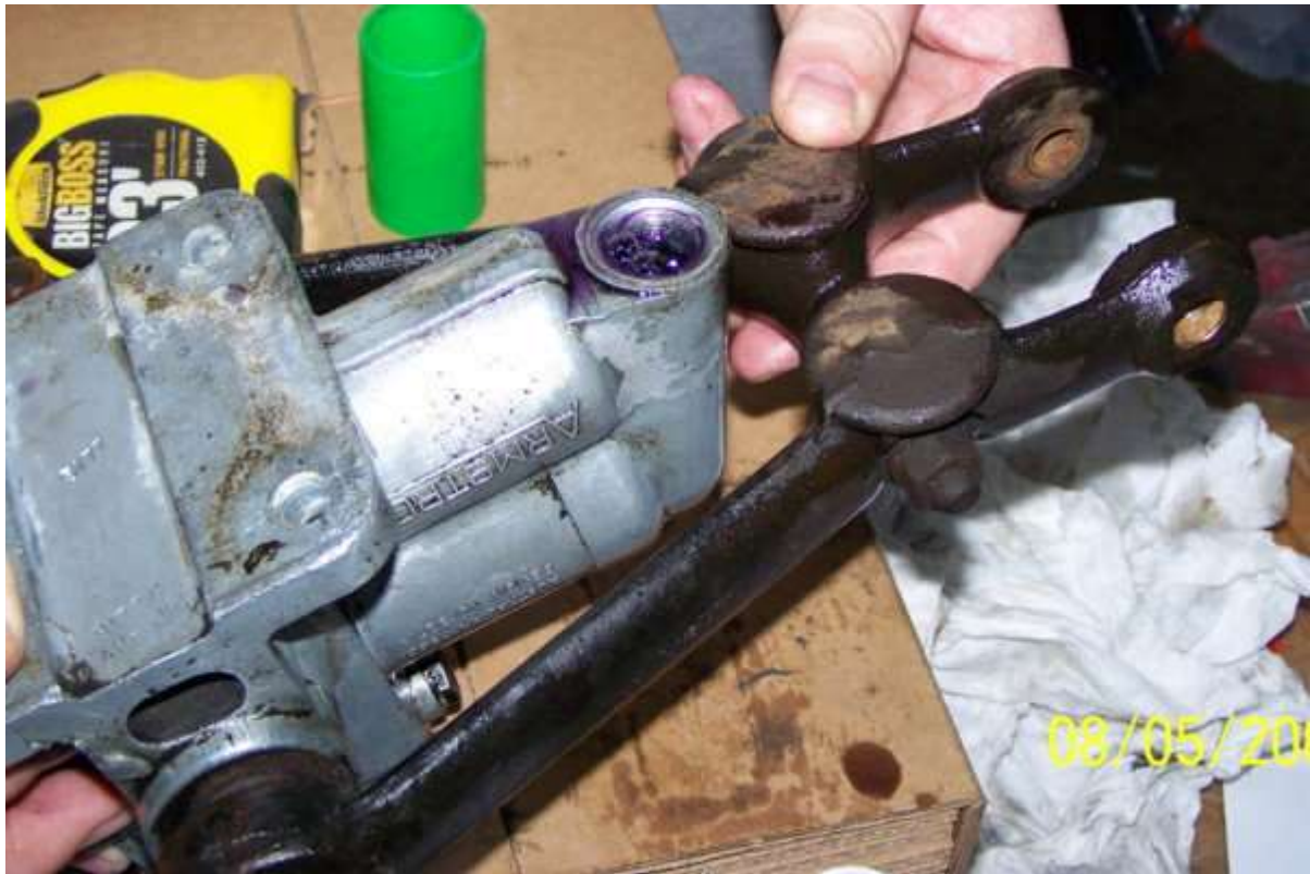
Working shock levers through full range
