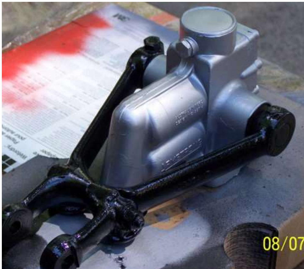
MGB Armstrong Lever Shock (Front), Refilled and Painted Like New
