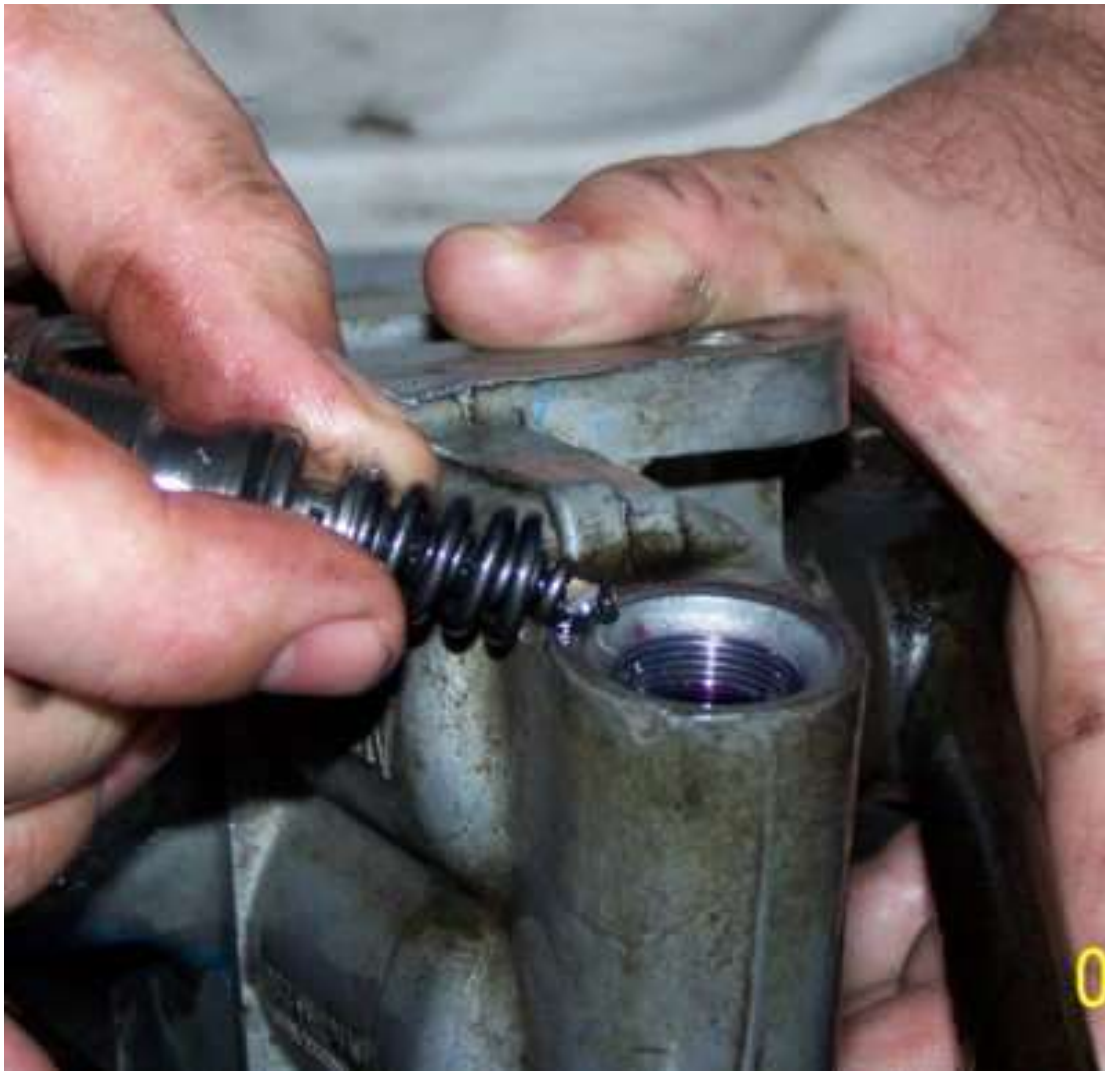
MGB Lever Shock valve assembly, removed. Here is a photo of the lever shock valve and piston assembly, courtesy of Peter Caldwell:
