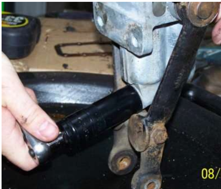
Removing MGB Lever Shock valve assembly
