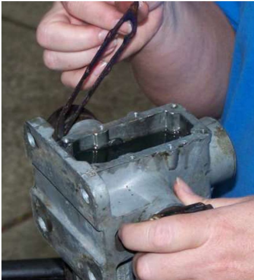
Removing MGB Lever Shock cover gasket
