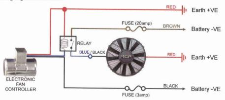
For safety reasons it is recommended that the vehicle battery is disconnected when you are carrying out this installation procedure.
