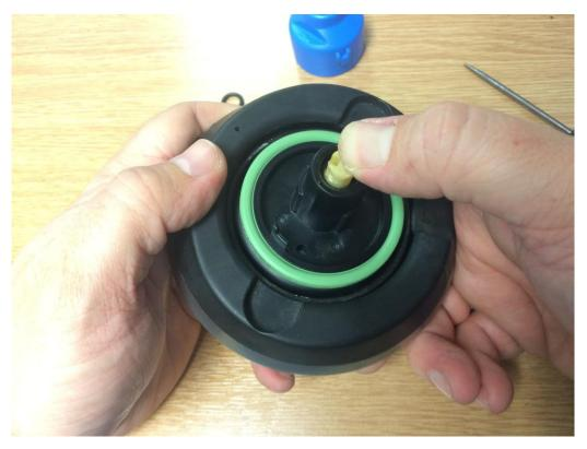
9. Leaving the key in the lock ensures that the barrel tumblers do not fall out of their locations.
