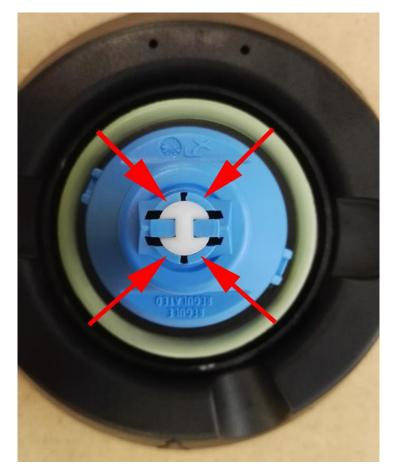
4. These four quadrants will need to be prised backwards to release the key barrel using a small flat bladed screw driver. They will need to be moved/bent back a considerable way to release their grip on the white central spindle
