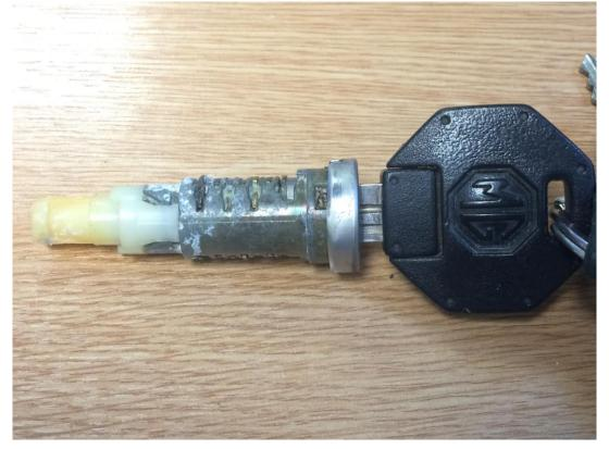
10. Remove the white spindle from the end of the barrel
