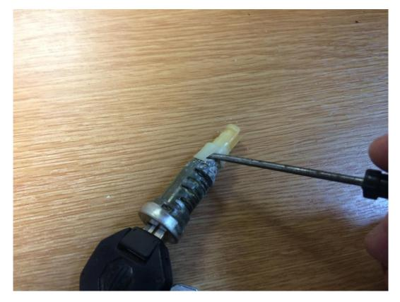
11. Clean up the barrel using suitable cleaning fluid & re-grease using a heavy moly or white grease.
