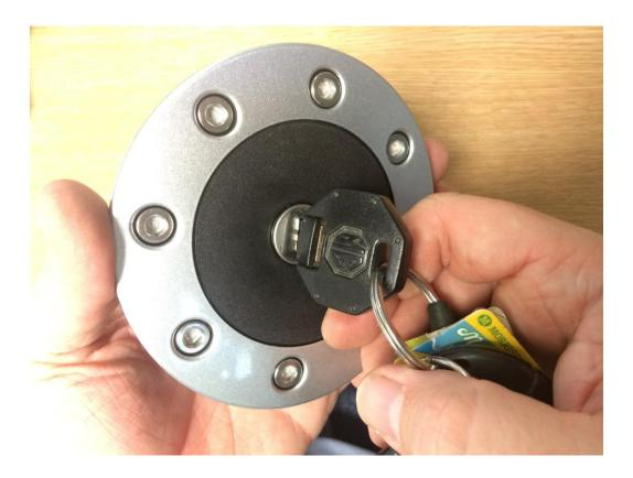
13. Smear a small amount of silicon grease to the green filler neck seal on the new filler cap and secure on the vehicle
