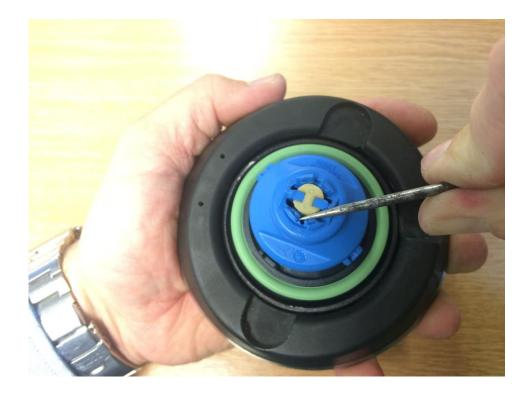
5. Once prised away pull the blue cap and it should lift clear of the filler cap.
