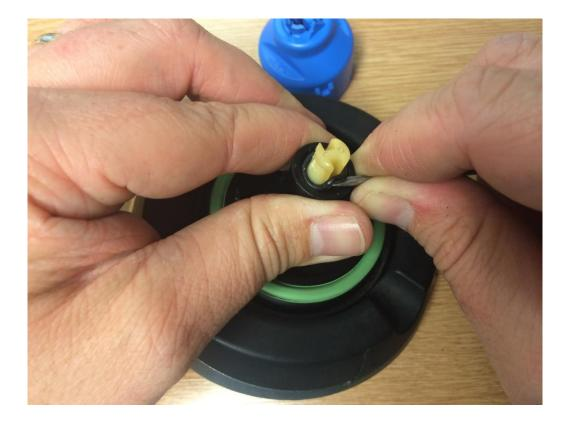
8. Holding the fuel cap in your hands, push down on the white spindle and the barrel will start to come out of the fuel cap.
