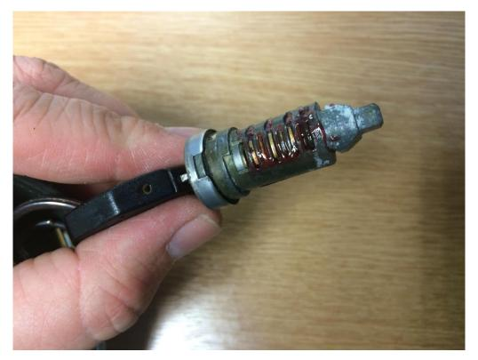
12. With your new fuel cap, push the barrel into the filler cap. It should locate firmly into place. You may need to turn it as you insert it into the new filler cap so that it is located properly in the locating lugs.
