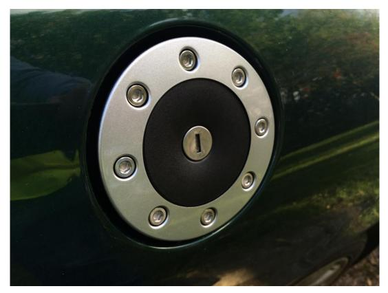
14. You may find the key is a little tight, over time the new seal will bed in to the filler neck and make for easier removal.
