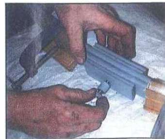
With spong leaves clamped, the centre bolt can be removed and the spacer shims filled
