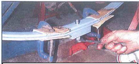
Here the shims are fitted below the spring giving maximum ride height
