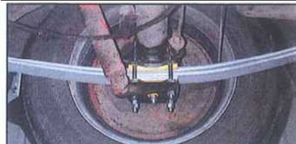
Complete installation showing telescopic shock absorber in position and visible clear gap between spring leaves
