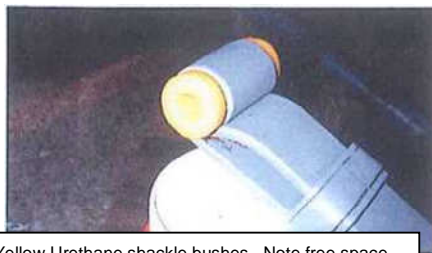
Yellow Urethane shackle bushes. Note free space between spring leaves
