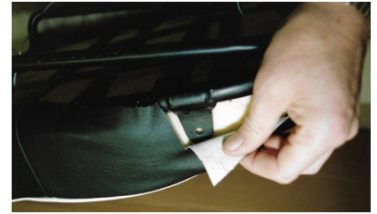
Pull the skirt over the frame & clip in place using tube clips. The skirt will need to be slit to pass around the pivot.
