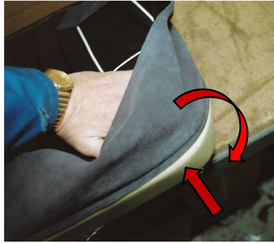
Place a hand inside the top of the cover, spread fingers along the piping, push the corner of the foam under the piping then roll the base skirt over the fingers & down the side of the foam & frame. Repeat for the other corner.
