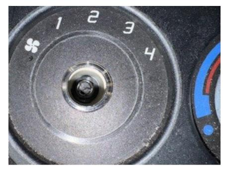
5. Line up the flat edge of the mortice at the rear of the alloy heater knob with the flat edge of the stem and slide the knob into place. The purpose of the grub screw is to provide engagement against the flat side of the heater control stem. A certain degree of adjustment if the grub screw is required to achieve sufficient engagement of the stem to retain the knobs in place.
