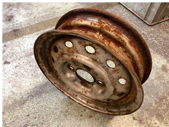
This wheel shows significant corrosion damage
