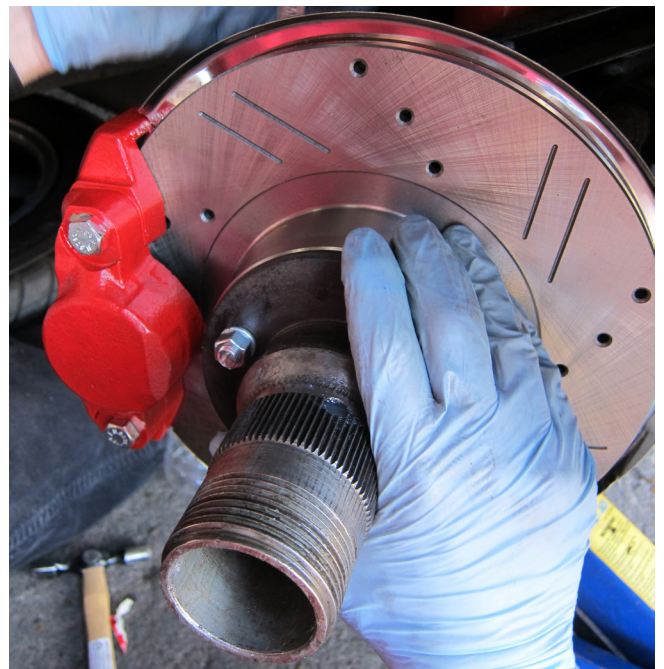
Having inspected the bearing end float, refit the hub assy. Using a new split pin, re-fit the caliper bending over the lock tabs to secure.
