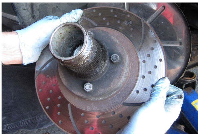
Remove grease cap, split pin and hub nut, then carefully set the hub assembly to one side.
