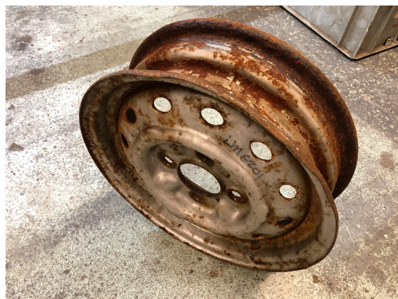
This wheel shows significant corrosion damage
