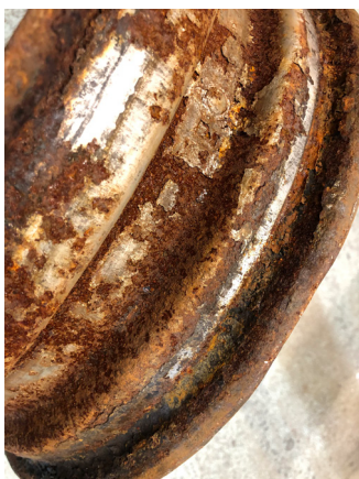
Note the bent rim on this wheel
