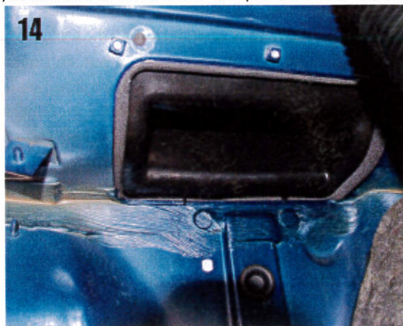
New air duct fitted, note hole in front is for the plastic cover trim as seen in image 15
