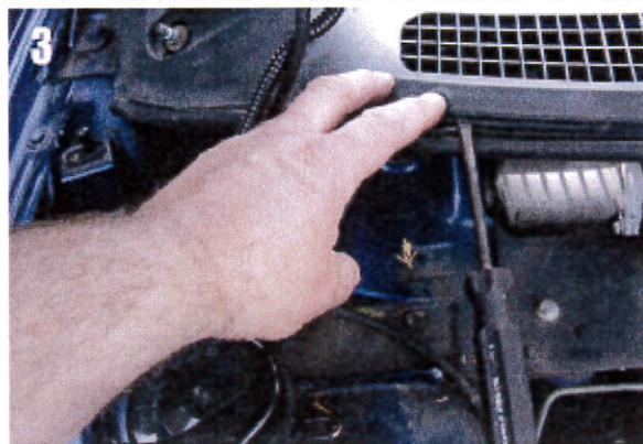
Removed screw cap and cross headed screw of which there are six to undo and extract
