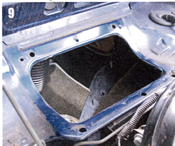
Quarter drive tools small enough to be more convenient to remove this front fixing
