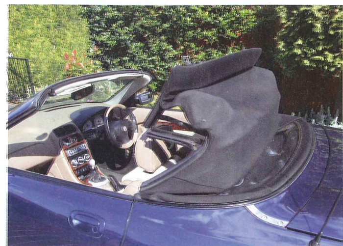
1 Typical Hood jammed in partial lowered position
