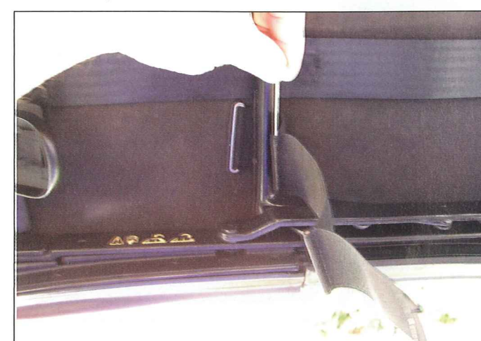
7 Feed an end of the new elastic strap around the stay and remove the steel pin from the pleat
