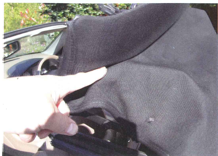
2 Finger pointing to the header rail jamming against the first hood cross stay
