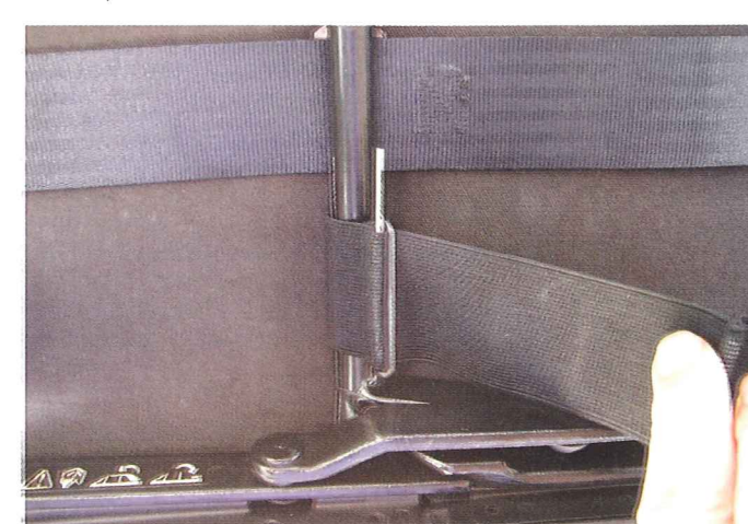
8 Squeeze and feed the pleat through the buckle at the end of the strap, then feed the steel pin back into the pleat
