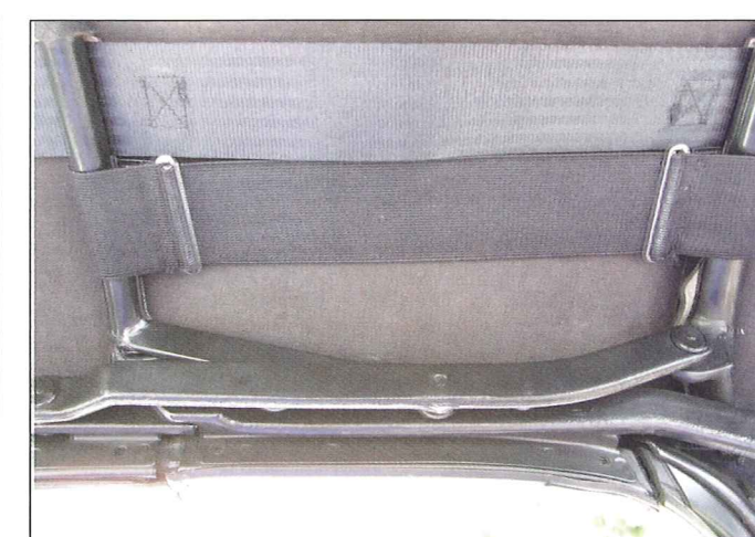
9 The assembled strap fitted to both hood stays
