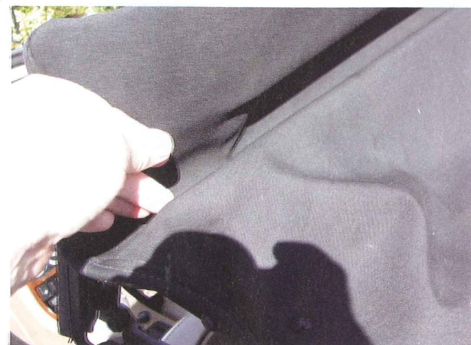
3 Even with a small manual movement of the first cross stay the hood lock is avoided
