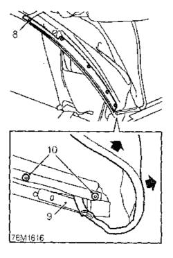
8. Remove 2 rivets securing ends of hood rear quarter retaining strips.
