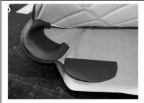
5: To prepare the squab covers for fitting, the half moon boards need to be replaced in their pockets at the bottom of the cover. These give the squab bottom something to screw into when finishing the squab fitting.
