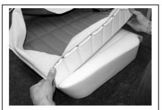
12: Before applying any glue it is necessary to dry fit the foam into the base frame, and this up with its corresponding squab cover, to make identical middle marks on the foam and base cover underside. When this is done the foam and cover can be glued as directed on the flat middle section. As before leave sufficient time for glue to set before proceeding.
