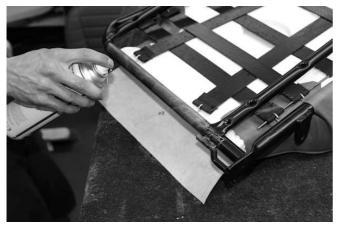
All that remains is to fix the squab assembly permanently to the base frame, and your newly re-trimmed seat can be returned to the car's interior.
