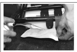
14: Finally with the skirt pulled down, slit approximately one inch at the point in front of the squab bolt hole brackets, and glue and tuck under the resulting flap of material.
