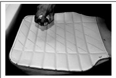
11: The base is attached to the frame using circular clips. You will see upon removing your old covers that the seat cover is glued into place on the foam by its middle, as shaded above. You may find it necessary to renew the diaphragm straps, which is most easily done by clamping the frame to a workbench and stretching them into position with a pair of pliers.
