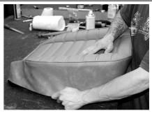
13: With the foam in position squarely on the frame, check again that the designs on squab and base line up correctly and that the front of the foam is flush with the frame. The skirt can now be rolled over the foam and pulled down to the base frame. Temporarily clip the sides and front of the skirt to test the fit of the cover on the frame.
