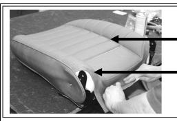
8: The area that needs to be glued follows the two vertical lines in the seat cover and foam, as indicated here with two arrows. Spray 2" of glue either side of these on both the cover and foam as accurately and as far inside the cover as you can. Support the cover and do not let the glued surfaces come into contact before the glue has been allowed to go tacky.
