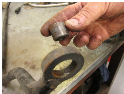
Removal of metalastic ARB bush
