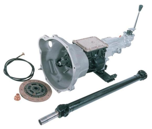
The MGA is an excellent road car and a driver's delight. One of the very few criticisms of this car on modern roads is its original gearbox and low overall gearing. The standard axle ratio of 4.3/1 gives 17 mph per 1000 rpm in 4th gear. These characteristics give a very lively performance right up to maximum speed. The major drawback is apparent when cruising on motorways at 70mph for long periods. The engine rpm at this speed is 4118 rpm which is high compared to modern vehicles with 5 gears.
