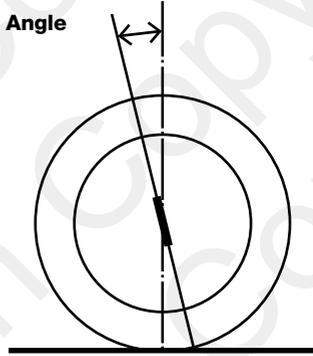
The Caster angle is the angle between the vertical and the inclination of the king pin when viewed from the side of the wheel
