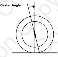
The Caster angle is the angle between the vertical and the inclination of the king pin when viewed from the side of the wheel
